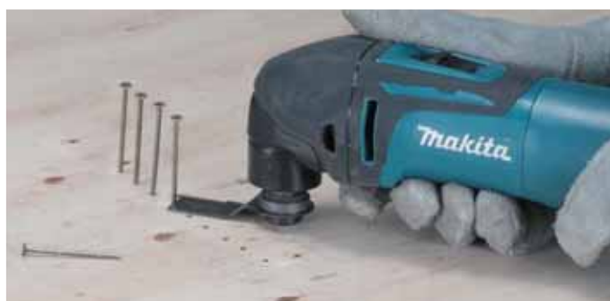
Flush cutting of nails
