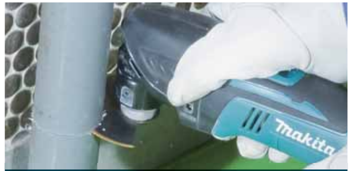
Cutting PVC, FRP pipes
